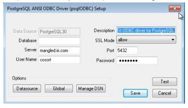
After your credentials are entered, test the connection by clicking on "Test" (make sure your VPN is running, if applicable).
